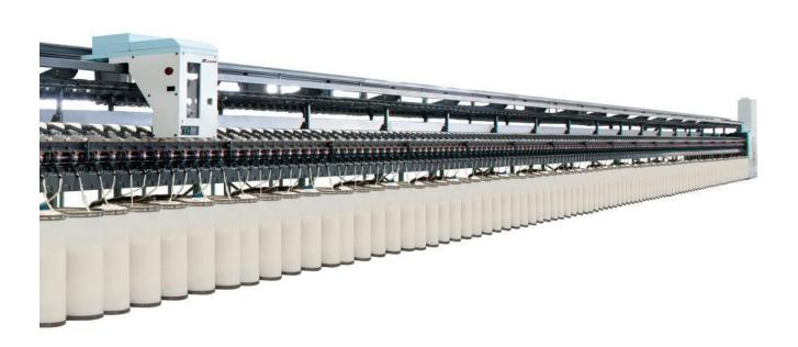
oMax spindles is up to 600 spindles, and the highest rotor design speed of 110000RPM. oModular design and abundant optional accessories to meet the needs of different customers. oInnovative auto doffing device can be as option, which increase production efficiency greatly. oMore electronic technology applications make machine smarter and more efficient.
